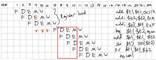
Show successful implementation of pipeline with clock cycles 8,9, and 10.
